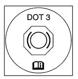
The brake master cylinder reservoir is filled with DOT-3 brake fluid. See Engine Compartment Overview on page 308 for the location of the reservoir.
